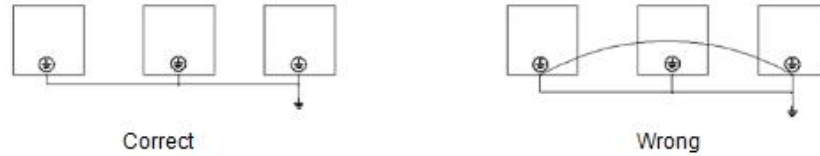
Figure 3-8 Grounding Wire Connection Sketch Map
